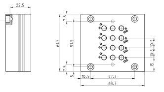
Note: the manifolds are supplied complete with the seals and the valves, fixing screws.
