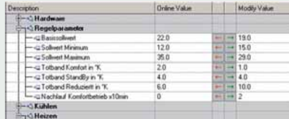
The control parameters (PI) for the specific applications can be adjusted and optimised.
