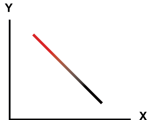
2-Axis Linear Interpolation
