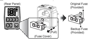
Replace the original fuse 1 with the provided backup fuse 2.
